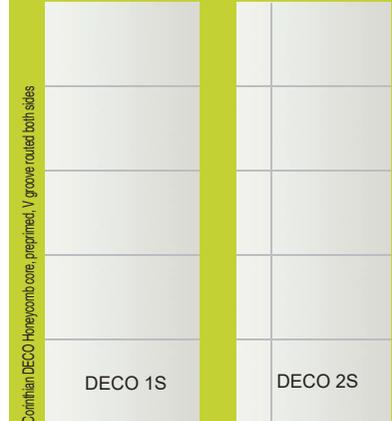
Corinthian DECO Honeycomb core, preprimed, V groove routed both sides
